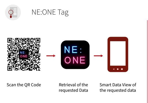
**NE:ONE Tag** forms the interface between the data available in ONE Record and the shop floor. This is software that can display and write existing data individually by process step at the piece level. This enables the automatic sharing of critical information via ONE Record.
