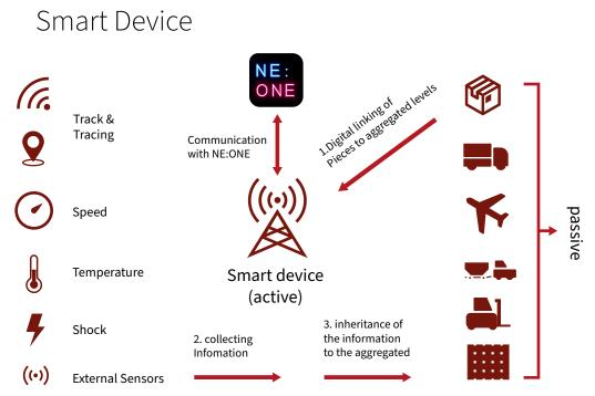
The **Smart-Device** connects the structure of various objects from reality via active and passive beacons and transfers them to the One Record data structure. This allows freight data, such as the current position, to be automatically transferred to a large number of consignments and actively shared.
